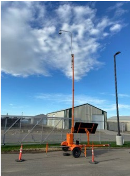
Existing Traffic Monitoring Trailer (Source: City of Williston)
