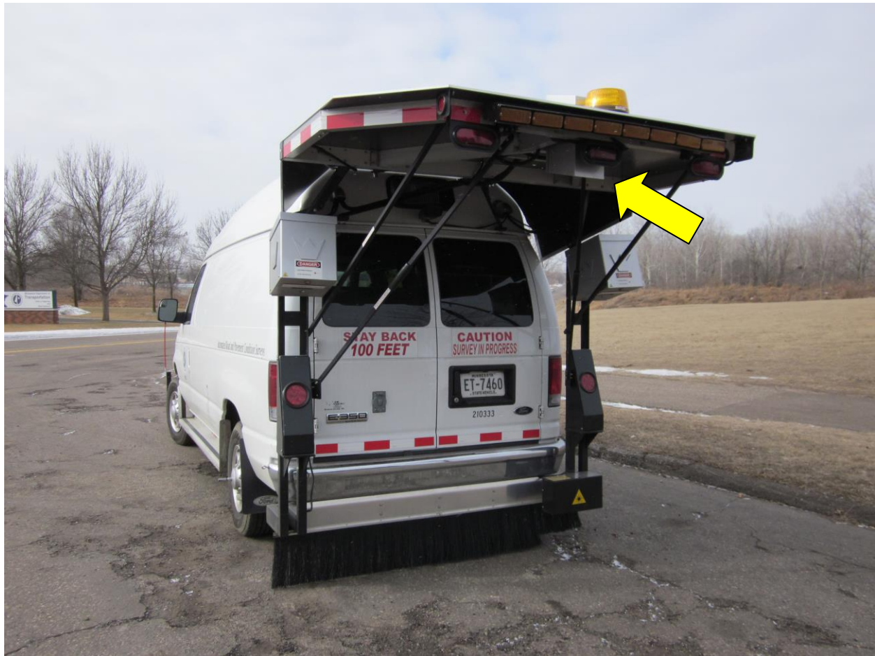
Figure 4. Close-up of 3D camera used to record pavement distress.
