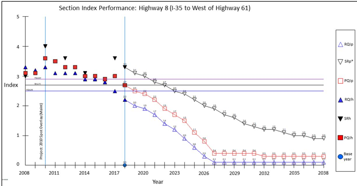
Figure 3.2 HPMA Pavement Performance Plot for Highway 8, West of Highway 61 to East of Greenway Avenue
