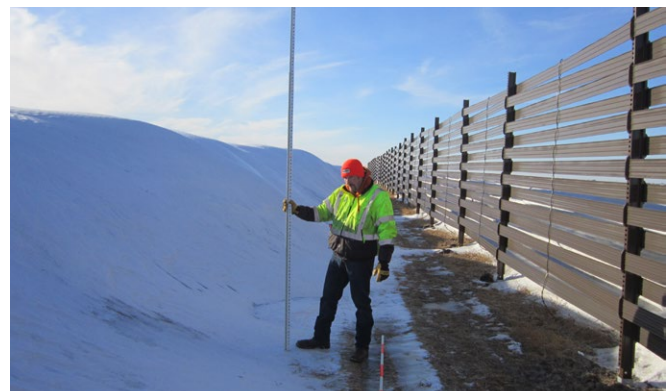
Eight foot snow drift behind a structural snow fence.
