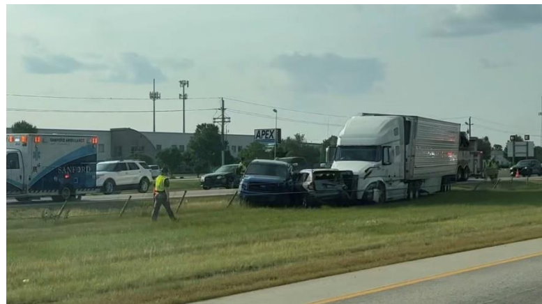
Figure 2. Semi, SUV, and Truck Crash Prevented from Crossing Median by HTMCG in Fargo (Valley News Live)
