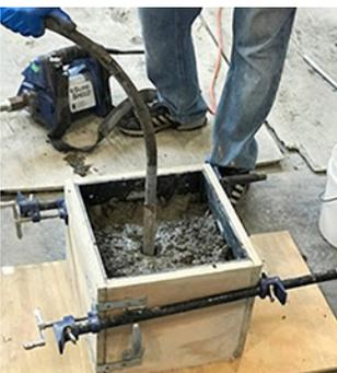
*The box test determines how well cement holds its form once hardened.*
