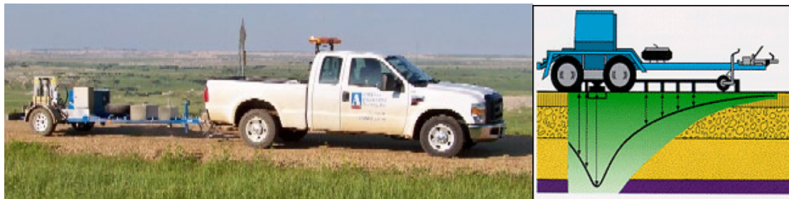
Figure C1 Dynatest 8002 FWD Test System
