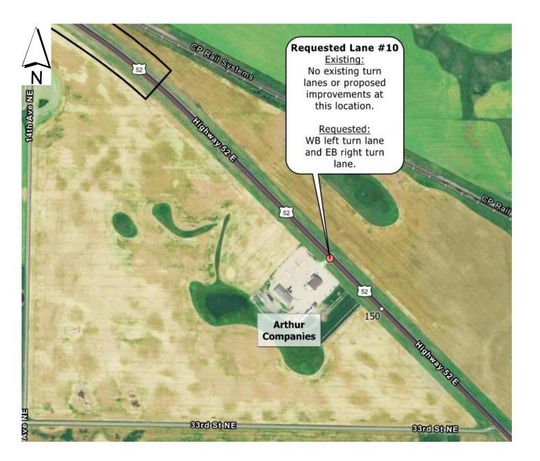
Note: The requested turn lane is not part of the INFRA Grant awarded to the NDDOT for this project. If a decision is made to install the requested turn lane, the turn lane will be designed and constructed as part of a separate project.
