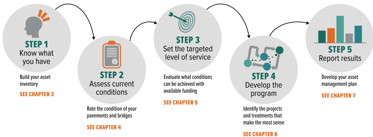
Figure 2-1. The steps in the TAM process. © 2017 Applied Pavement Technology, Inc.
