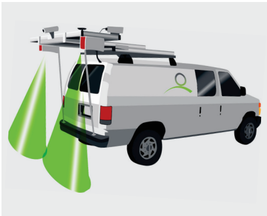
Figure 4–2. Illustration of automated data collection equipment © 2017 Applied Pavement Technology, Inc.
