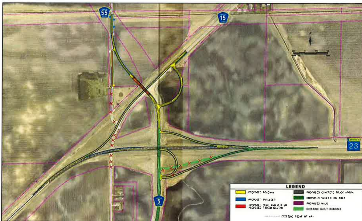
Figure 8 – Alternative 4 - Folded Diamond Interchange B Layout
