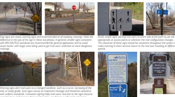
Stop signs are classic warning signs and recommended at all roadway crossings. Note the difference in the size of the sign in these two photos. In general, smaller signs consistent with MN MUTCD standards are recommended for general application and to avoid visual clutter, with larger ones being used to get trail users' attention at more dangerous crossings.
