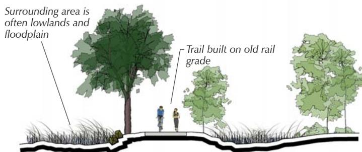
**Primary Trail Route** – after crossing County Rd. 18, the trail essentially follows an old rail grade, which will require regrading, culvert replacement, and a few bridges to make it suitable for developing the trail.
