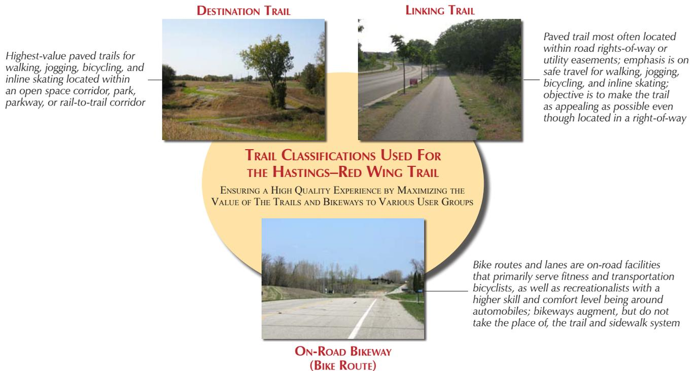
With the Hastings–Red Wing Trail, the goal is to maximize the use of “destination” trails since these offer the highest overall recreational value. Where “linking” trails are used (such as along Ravenna Trail Road), minimizing impediments to travel and maximizing the appeal of the corridor are important to encouraging high use levels of use for recreation, fitness, and transportation.
