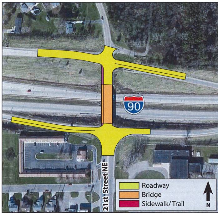
Figure 22. 21st Street NE Interchange Bridge Replacement Concept
