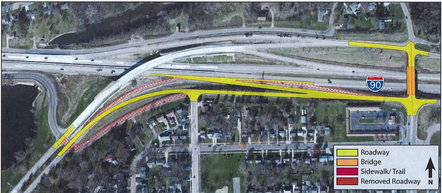
Figure 26. Oakland Place Interchange Reconfiguration Concept
