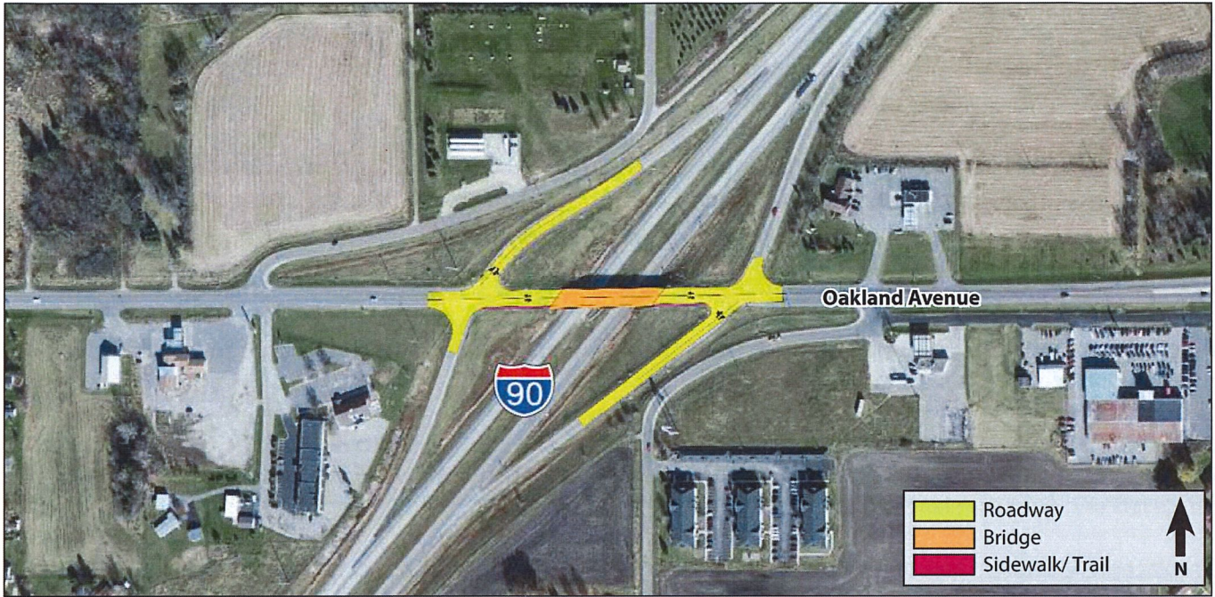
Figure 9. TH 105/Oakland Avenue Interchange Bridge Replacement Concept
