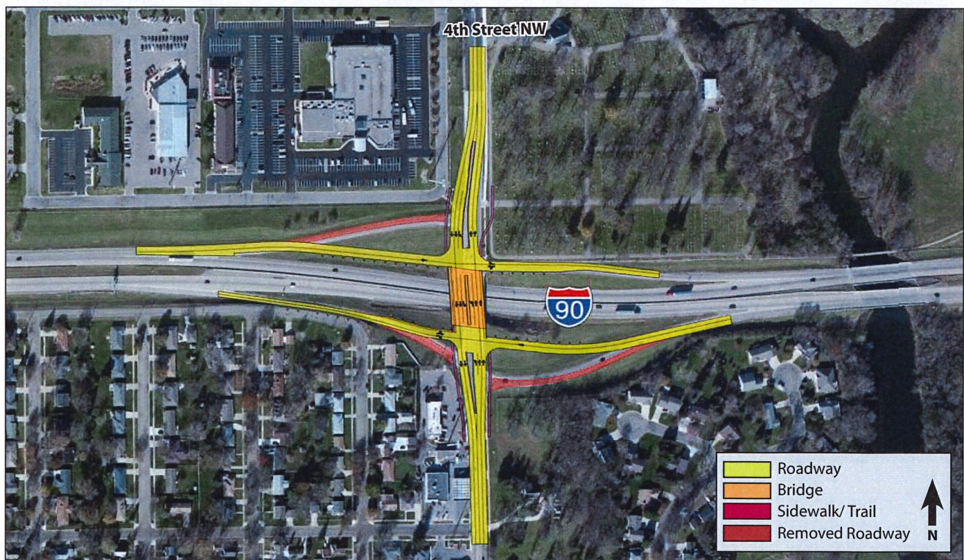
Figure 14. 4th Street NW Interchange Reconstructed Diamond Concept
