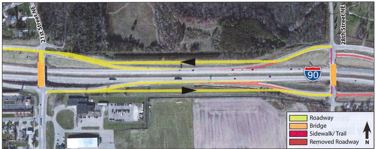
Figure 20. 21st Street NE and 28th Street NE Interchanges: One-way Frontage Road Concept
