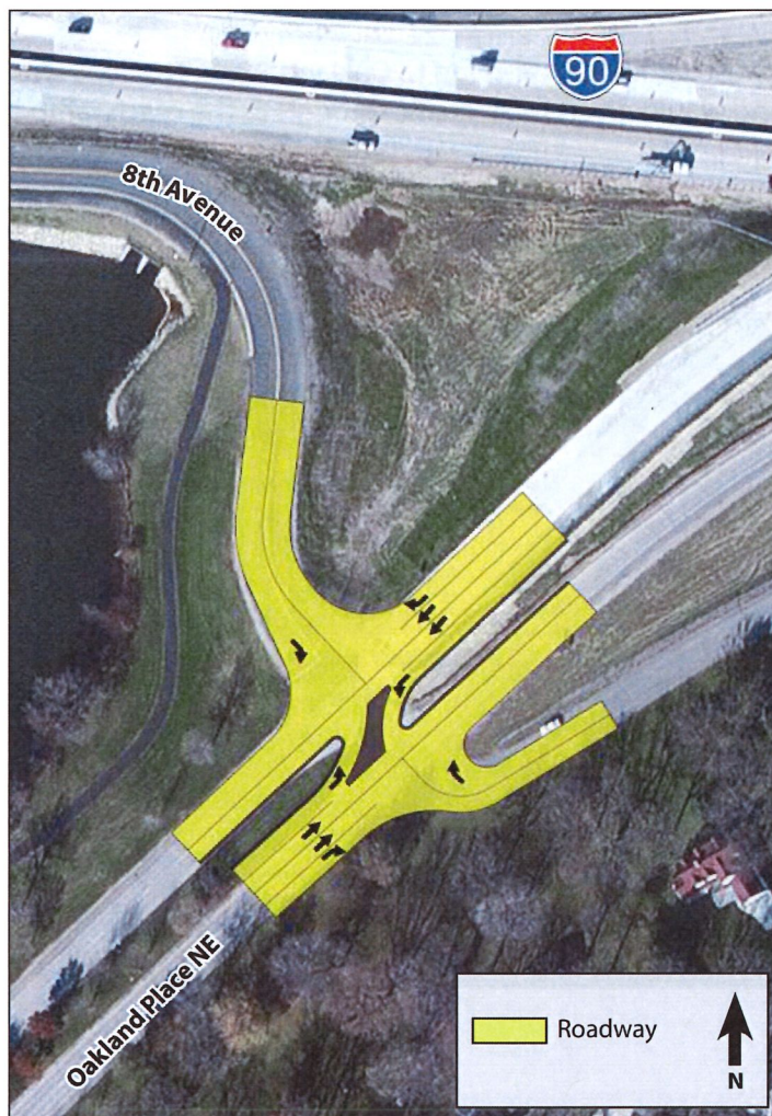
Figure 27. Oakland Place/8th Avenue \frac{3}{4} Access Intersection Concept
