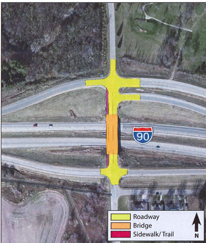
Figure 24. 28th Street NE Interchange Bridge Replacement Concept
