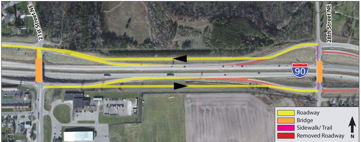
Figure 20. 21st Street NE and 28th Street NE Interchanges: One-way Frontage Road Concept
