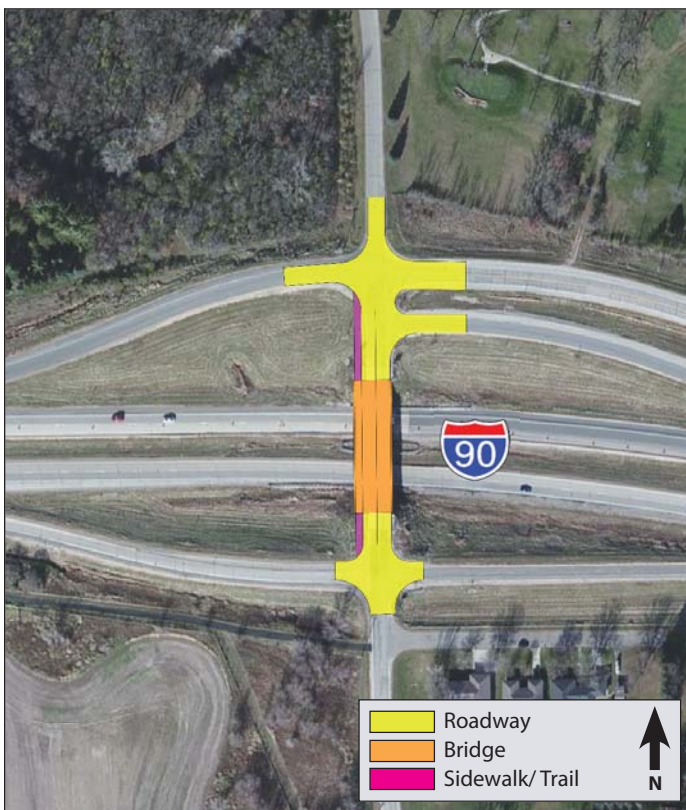
Figure 24. 28th Street NE Interchange Bridge Replacement Concept
