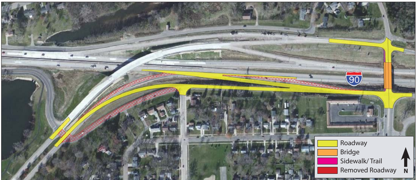
Figure 26. Oakland Place Interchange Reconfiguration Concept
