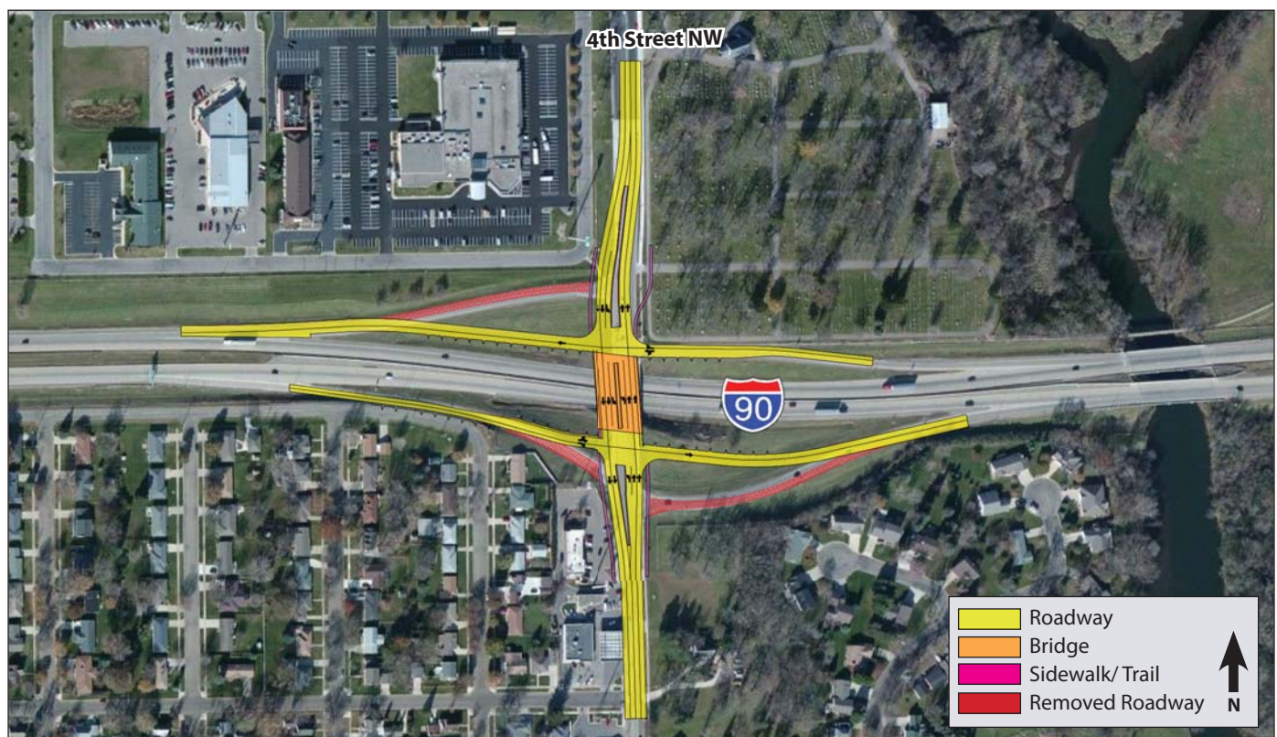
Figure 14. 4th Street NW Interchange Reconstructed Diamond Concept
