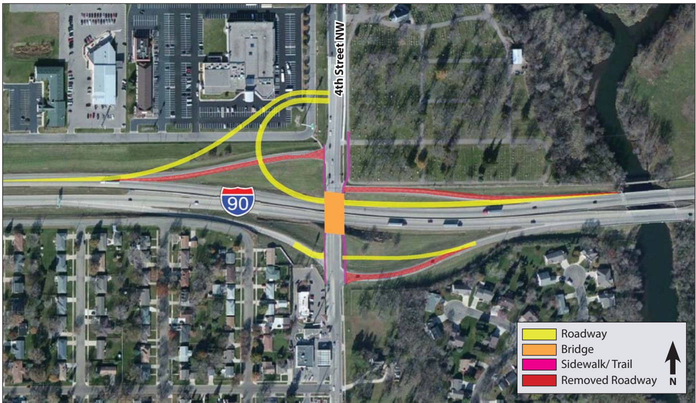
Figure 17. 4th Street NW Interchange Folded Loop Concept
