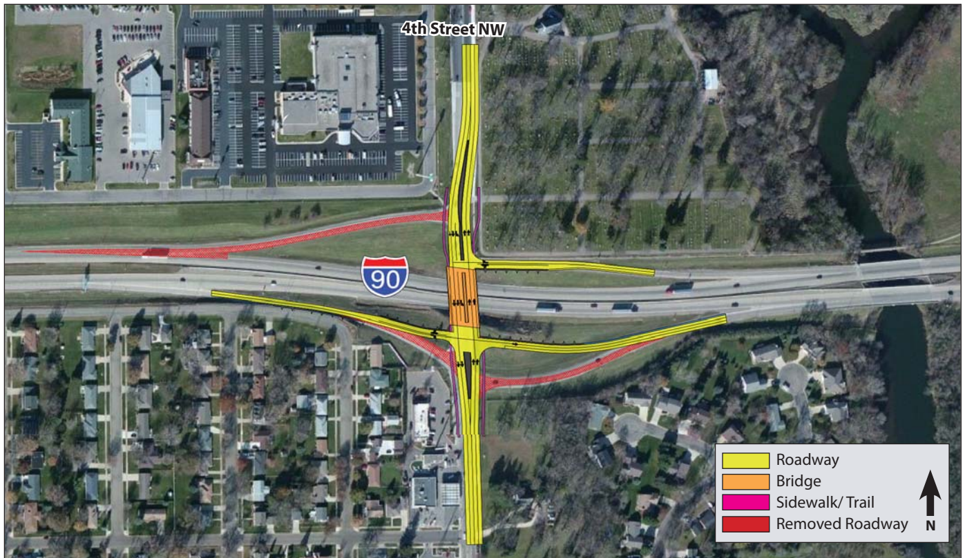
Figure 15. 4th Street NW Interchange Partial Diamond Concept
