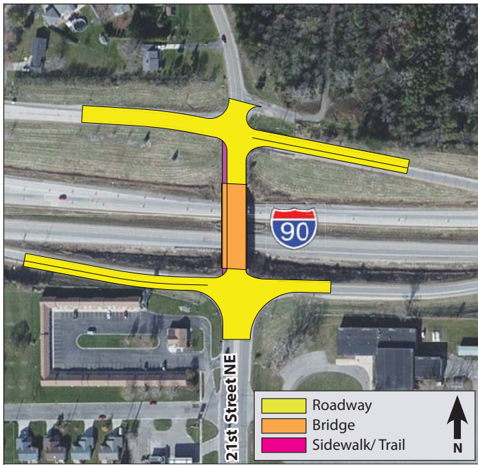
Figure 22. 21st Street NE Interchange Bridge Replacement Concept
