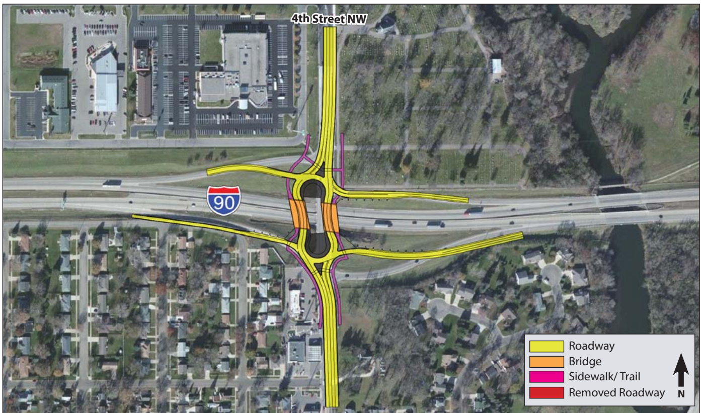
Figure 16. 4th Street NW Interchange Roundabout Concept
