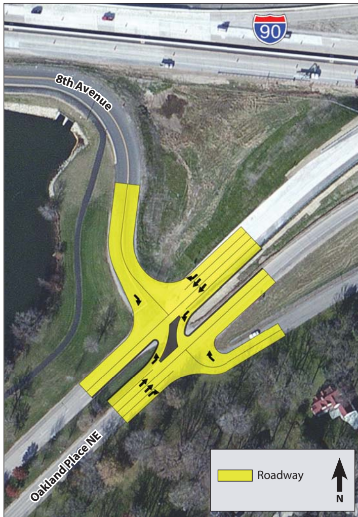
Figure 27. Oakland Place/8th Avenue \frac{3}{4} Access Intersection Concept
