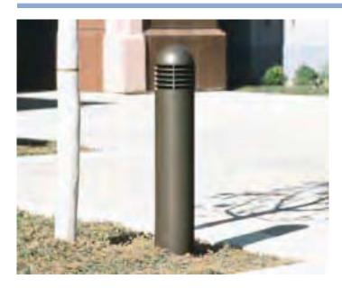
**Top Cap:** One-piece aluminum casting 3/6° minimum thickness, secured to louvers by concealed allen screws in keyhole slots. For relamping access, allen screws shall not require complete removal.
