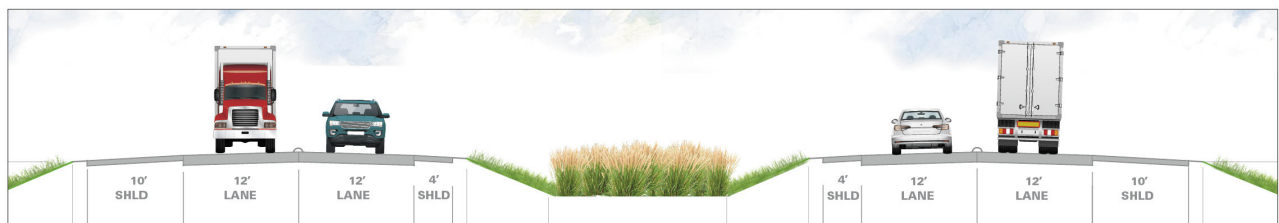
10 Miles of 2-lane to 4-lane expansion
