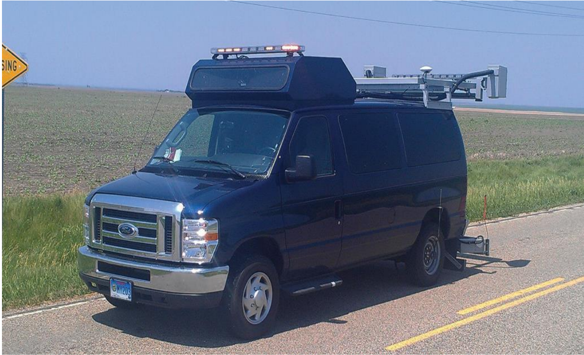
Figure 3.10: Road and Pavement Data Collection Vehicle
